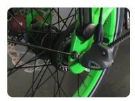
Internal Nexus 3 Speed Hub and Bell Crank
