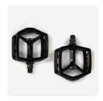
Using the 15 mm wrench provided in the tool kit, attach and tighten the pedals. PLEASE NOTE – The pedals are marked "L" for Left and "R" for Right. The left pedal is attached by turning it counterclockwise and the right pedal is tightened by turning it clockwise. Make sure the pedals are tightly attached to the crank arms to prevent stripping.
