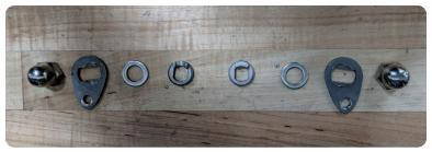
Orientation of hardware for front wheel assembly
