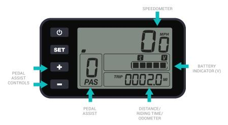
Press the power button (top button) on the four button selector located near the left grip on the handlebars to turn the meter on. You can adjust the pedal assist power level to have more power by hitting the [+] button (third button) and can move to a lower level power by hitting the [-] button (fourth button).
