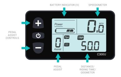
Press the power button [o] on the three button selector located near the left grip on the handlebars to turn the meter on. You can adjust the pedal assist power level to have more power by hitting the [+] button (top button) and can move to a lower level power by hitting the [-] button (bottom button).
