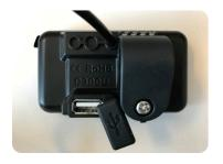
Each meter has an integrated USB port located underneath to charge your mobile devices. Press and hold [�] & [+] for 2 seconds to turn on the USB charge function; press and hold [�] & [+] for 2 seconds to turn the USB charge function off.
