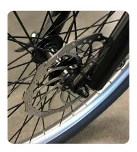
Your Pedego is equipped with hydraulic disc brakes for maximum reliability. Applying hand pressure to the brake levers will engage the brake pads against the brake rotor, creating friction and slowing down the wheel. The more hand pressure applied to the brake lever, the faster the bike will come to a stop.
