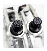
Using the 15 mm wrench provided in the tool kit, attach and tighten the pedals. PLEASE NOTE – The pedals are marked "L" for Left and "R" for Right. The left pedal is attached by turning it counterclockwise and the right pedal is tightened by turning it clockwise. Make sure the pedals are tightly attached to the crank arms to prevent stripping.
