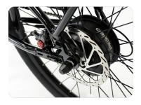
Your Pedego is equipped with disc brakes for maximum reliability. Applying hand pressure to the brake levers will engage the brake pads against the brake rotor, creating friction and slowing down the wheel. The more hand pressure applied to the brake lever, the faster the bike will come to a stop.
